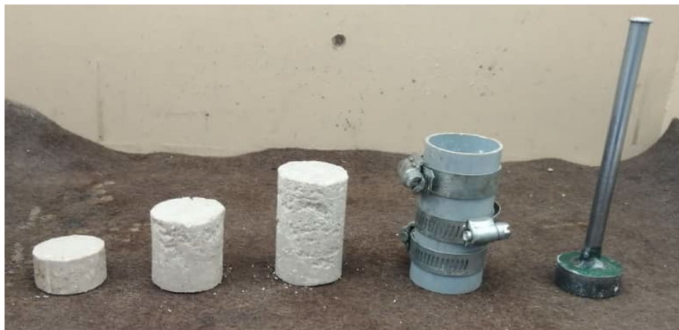
Fig. 4 The prepared samples with bentonite base with 15, 30, and 45% of hematite powder in heights of 2, 4, and 6 cm
